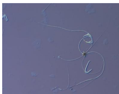
Double Wall Nanotube Bundles Diameter less than 10nm – Image size: 160 \mu\text{m}
